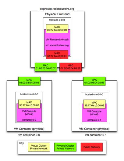
In the above picture, "espresso.rocksclusters.org" is a physical machine. Also, "vm-container-0-0" and "vm-container-0-1" are physical machines that were kickstarted by "espresso". The machine "frontend-0-0-0" is a virtual machine that is hosted by "espresso". The machines "hosted-vm-0-0-0" and "hosted-vm-0-1-0" are VMs that are associated with "frontend-0-0-0" (they are all in the same VLAN).
