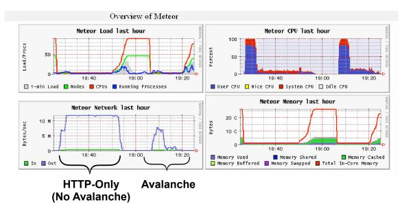
Figure 2: Without Avalanche (start time: 18:25), the full cluster re-installation takes more than 30 minutes. With Avalanche (start time: 19:05) takes less than 20 minutes for all nodes to complete. Note the reduction in network traffic directed to the Meteor Frontend when Avalanche is active. Meteor's frontend is an 800 MHz PIII with 100Mbit Ethernet.
